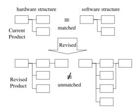
Fig. 2 Inconsistency between hardware and software structures.
