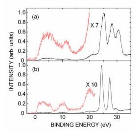
Figure 4 XPS spectra of (a) e-BGO and (b) s-BGO.
