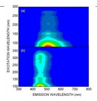
**Figure 2** Contour plot of the 3D emission-excitation spectra of (a) e-BGO and (b) s-BGO at T = 5 K.
