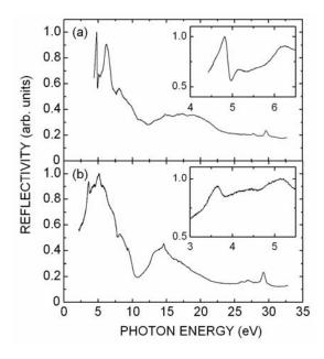
**Figure 1** Reflection spectra of (a) e-BGO and (b) s-BGO at T = 5 K. The insets show the low-energy part in an expanded scale.
