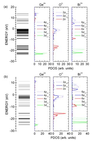
**Figure 5** Energy diagrams and PDOS curves of (a) e-BGO and (b) s-BGO calculated by the DV- $X\alpha$  method.
