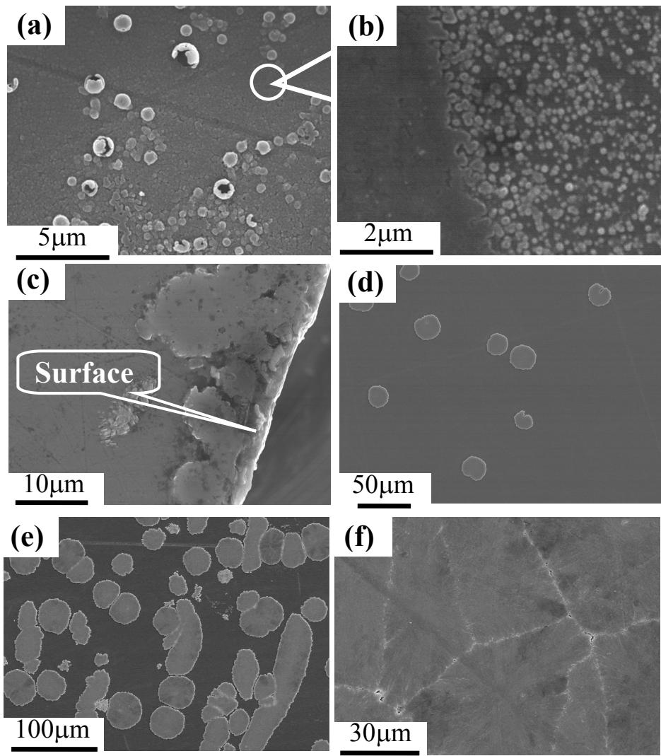
**Fig. 1.** SEM photographs of polished and chemically etched surfaces of the Ca06 parent glass at (a) low magnification and (b) high magnification, (c) near the surface and (d) deep inside of the Ca06 specimen heated at 770°C for 2 h, and (e) and (f) deep inside of the Ca06 specimen heated for 2 hours at 800°C and 850°C respectively. The “Surface” shown in the figure is the original surface of the specimen which was not polished.
