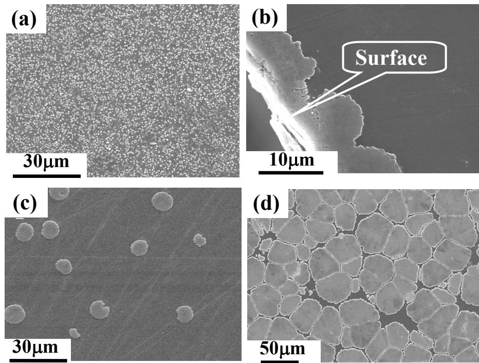
**Fig. 2.** SEM photographs of polished and chemically etched surfaces of (a) the CaK001 parent glass, (b) near the surface and (c) deep inside of the CaK001 specimen heated at 740°C for 2 h, and (d) deep inside of the CaK001 specimen heated at 780°C for 2 h. The “Surface” shown in the figure is the original surface of the specimen which was not polished.
