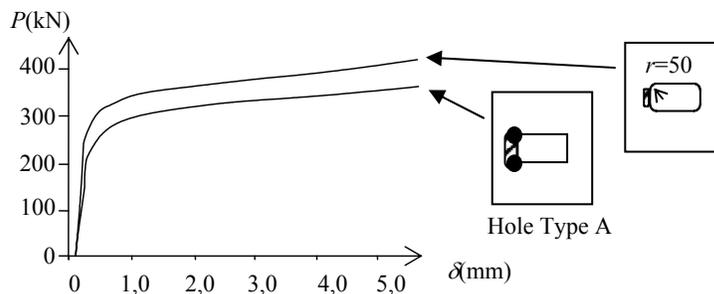
Fig. 14. Effect of Rounded Hole Corner
