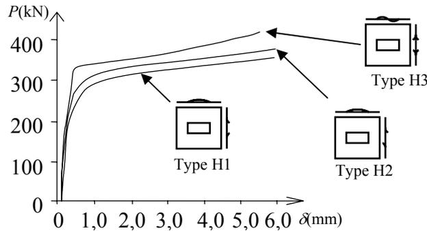
Fig. 12 Load-Deflection Curves of Initial Deflection Type H
