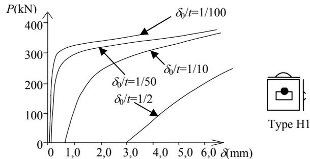
Fig. 10. Load-Deflection Relations according to Initial Deflection
