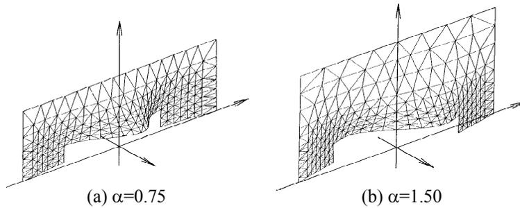
Fig. 6. Buckling Mode of the Hole Type A
