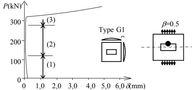
Fig. 11. Typical Load-Deflection curves
