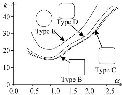
Fig. 8 Buckling Coefficients of Hole Types B-E
