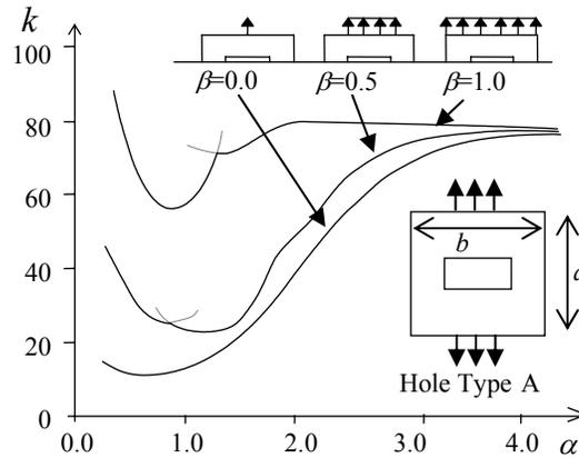
Fig. 7 Buckling Coefficients-Aspect Ratio Curves of Hole Types A
