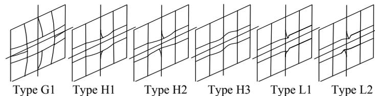
Fig. 9 Initial Out-of-Plane Deformation Patterns
