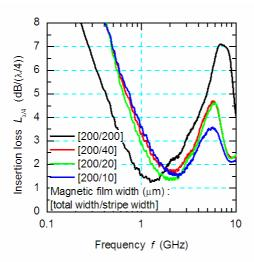
FIG. 6 The frequency dependence of insertion loss per a quarter wavelength  $L_{\lambda/4}$  of the fabricated device. The labels are similar to Fig. 4.
