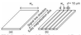
FIG. 2 Structure of the magnetic film. (a) Continuous magnetic film and (b) slit-patterned magnetic film.
