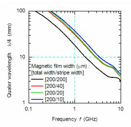
FIG. 5 The frequency dependence of quarter wavelength  $\lambda/4$  of the fabricated device. The labels are similar to Fig. 4.
