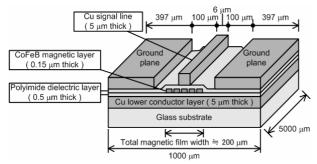
FIG. 1 Structure of the fabricated hybrid thin-film coplanar-line.
