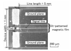
FIG. 3 Photograph of the fabricated hybrid thin-film coplanar-line with 10 µm wide magnetic film stripes.
