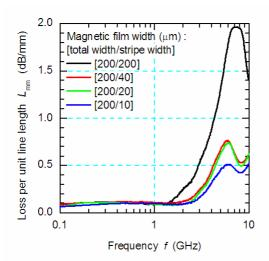
FIG. 4 The frequency dependences of loss per unit line length  $L_{mm}$  of the fabricated devices. The labels show total width and stripe width of magnetic film.
