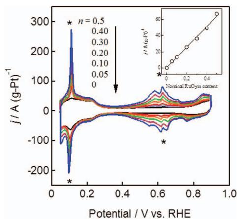
**Figure 4.** Cyclic voltammograms of RuO<sub>2</sub>ns(*n*)-Pt/C, with *n* = 0 to 0.5 at 50 mV s<sup>-1</sup> in 0.5 M H<sub>2</sub>SO<sub>4</sub>(60°C).
