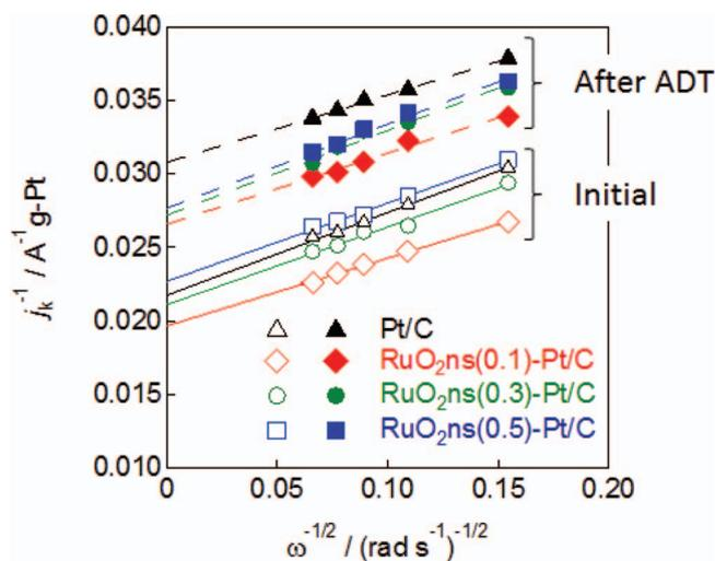
**Figure 6.** Koutecky-Levich plots of Pt/C and RuO<sub>2</sub>ns-Pt/C before (open markers) and after durability test (filled markers) at 0.90 V vs. RHE.
