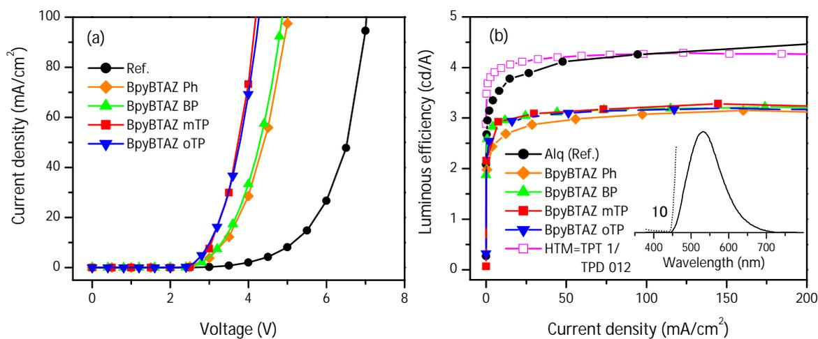
Figure 6. (a) Current density–voltage ( $J$ – $V$ ) and (b) luminous efficiency–current density ( $-J$ ) curves of devices with each BpyBTAZ. The inset in panel (b) shows the EL spectrum of the BpyBTAZ-mTP device and the dotted line is a  $\times 10$  magnification.
