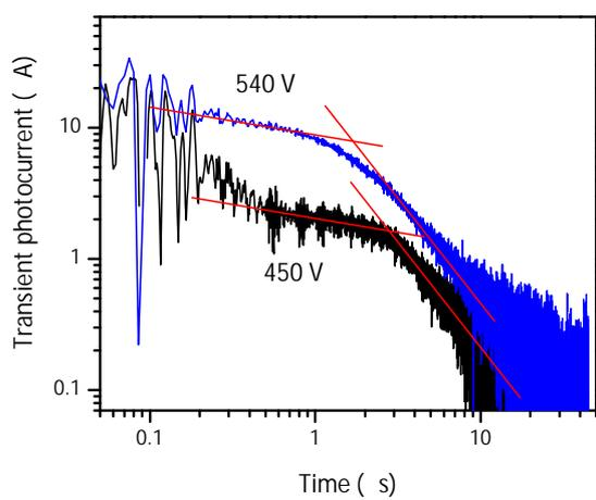
Figure 7. Transient photocurrent curves of TOF measurement of BpyBTAZ-mTP at the applied voltages of 450 and 540 V. Red straight lines are drawn to help determine the transit time.
