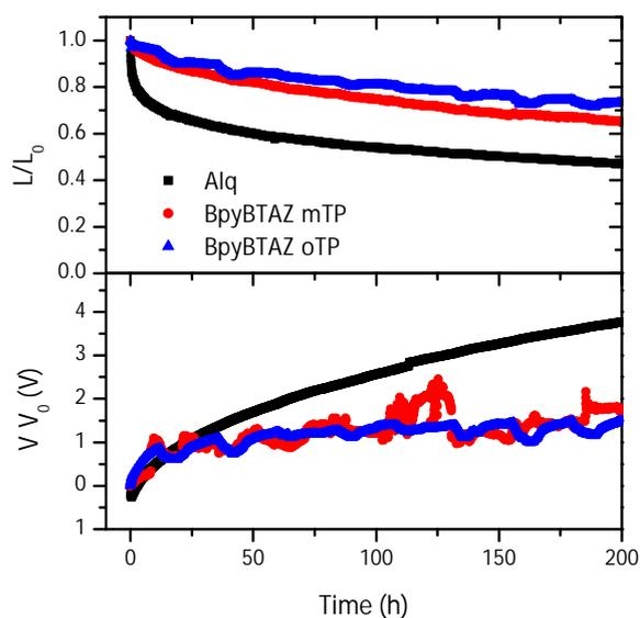
Figure 9. Luminance and voltage changes under constant current density operation at 50 mA/cm<sup>2</sup> for devices with different ETMs. The device structure is the same as the test OLED shown in Fig. 2. The devices were encapsulated by a glass cap with fresh desiccant using UV glue in an inert glove box (O<sub>2</sub> < 5 ppm, dewpoint < -50 °C).
