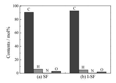
**Fig. 4.** Elemental composition of carbon fibers prepared from untreated and iodinated SF carbonized at 1400 °C for 12h: (a) untreated specimen, (b) iodinated specimen.
