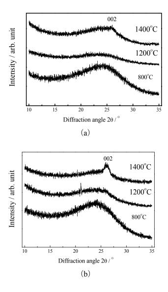
**Fig. 1.** Equatorial WAXD profiles of carbon fibers prepared from untreated and iodinated SF carbonized at 1400 °C for 12h: (a) untreated specimen, (b) iodinated specimen.
