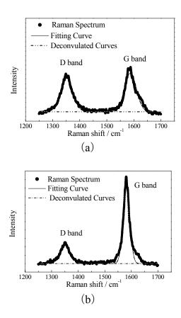
**Fig. 2.** Raman spectra of carbon fibers prepared from untreated and iodinated SF carbonized at 1400 °C for 12h: (a) untreated specimen, (b) iodinated specimen.
