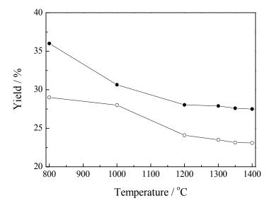
**Fig. 5.** Carbon yield of untreated and iodinated SF fibers obtained at different heating temperature: (○) untreated specimen, (●) iodinated specimen.
