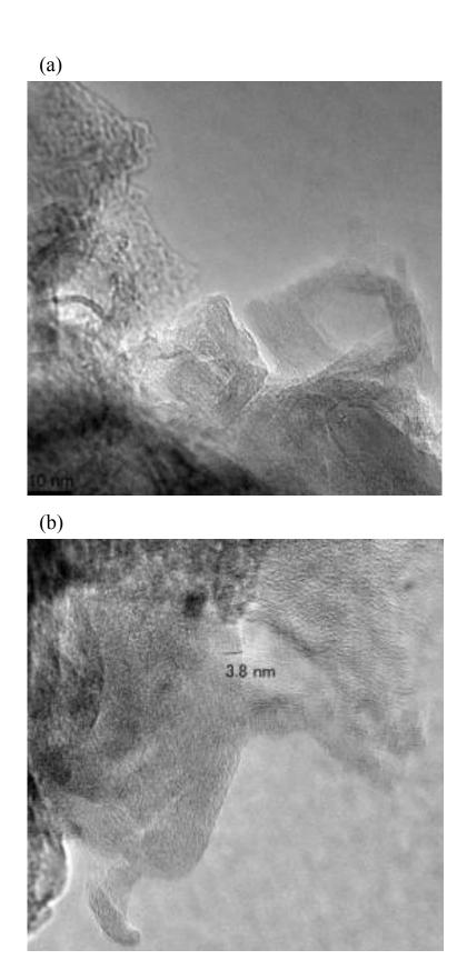
**Fig. 3.** TEM images of carbon fibers prepared from untreated and iodinated SF carbonized at 1400 °C for 12h: (a) untreated specimen, (b) iodinated specimen.
