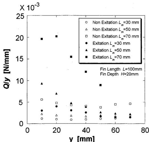
Fig. 5 Bending force per deflection of the fin
