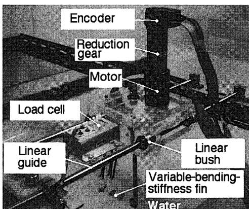
Fig. 6 Photograph of propulsion mechanism
