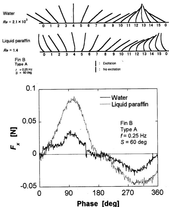
Fig. 12 Change in fin shape and variation of  $x$ -directional thrust force  $F_x$  for one movement cycle for water and liquid paraffin
