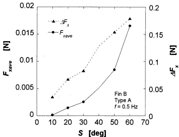
Fig. 10 Average thrust force  $F_{xave}$  and thrust force difference  $\Delta F_x (=F_{xmax} - F_{xmin})$  versus swing angle  $S$
