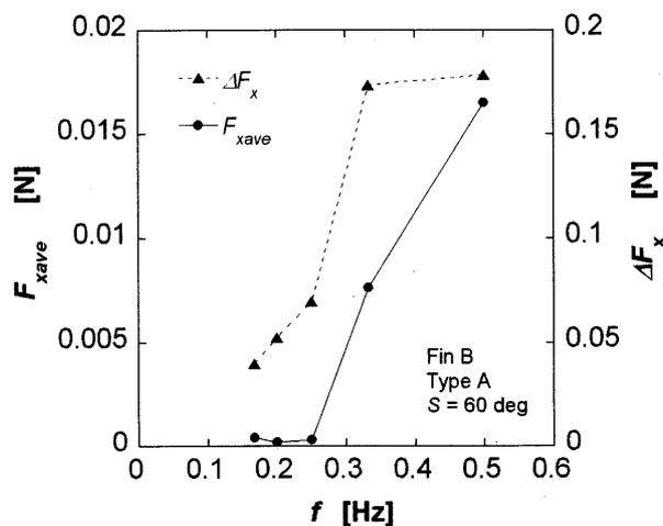
Fig. 9 Average thrust force  $F_{xave}$  and thrust force difference  $\Delta F_x (=F_{xmax} - F_{xmin})$  versus movement frequency  $f$
