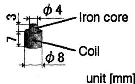
Fig. 3 Schematic of electromagnet
