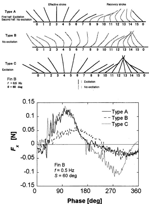
Fig. 8 Change in fin shape and variation of  $x$ -directional thrust force  $F_x$  for one movement cycle
