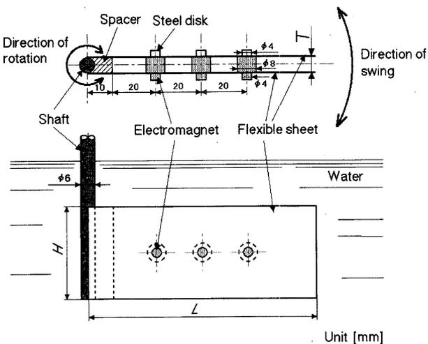
Fig. 1 Structure of variable-bending-stiffness fin
