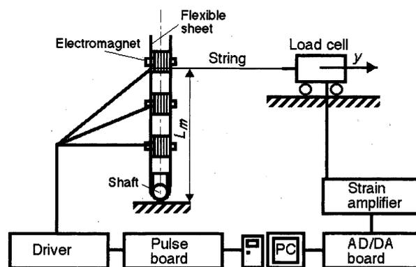
Fig. 4 Measurement system for fin's bending force and deflection
