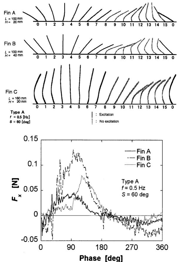
Fig. 11 Change in fin shape and variation of  $x$ -directional thrust force  $F_x$  for one movement cycle for the three fins of different sizes
