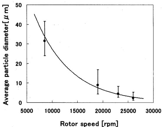
Fig. 3 Relationship between rotor speed of homogenizer and average particle diameter (Homogenizing time: 300 s). Error bars show standard deviation based on logscale particle diameter distribution
