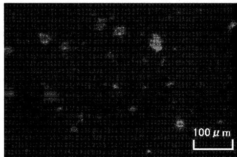
Fig. 5 Confocal microscope image of protein particles in distilled water (Homogenizing time: 300 s, Rotor speed: 19 000 rpm)
