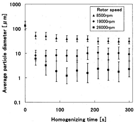
Fig. 2 Relationship between homogenizing time and average particle diameter. Error bars show standard deviation based on logscale particle diameter distribution
