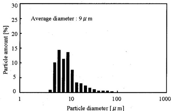
Fig. 4 Particle diameter distribution of suspension (Homogenizing time: 300 s, Rotor speed: 19 000 rpm)
