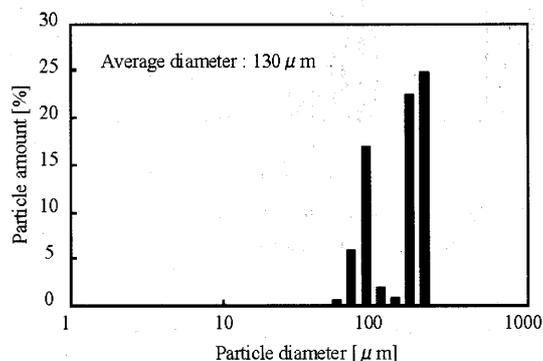
Fig. 1 Particle diameter distribution of suspension (Homogenizing time: 5 s, Rotor speed: 8 500 rpm)
