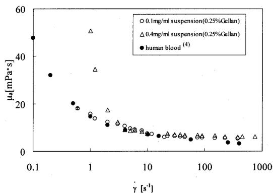
(b) Carrier fluid: 0.25 wt% gellan solution
