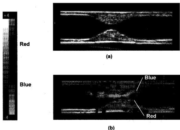
Fig. 10 Ultrasound image of the model with perfusion of the suspension. Steady flow, flow rate: 6 mL/s, probe: linear (7.5 MHz). Flow: Right  $\rightarrow$  Left. (a) B-mode. (b) Color Doppler mode: blue represents downward flow, red represents upward flow; color bar shows velocity of flow ( $\pm 4$  m/s)
