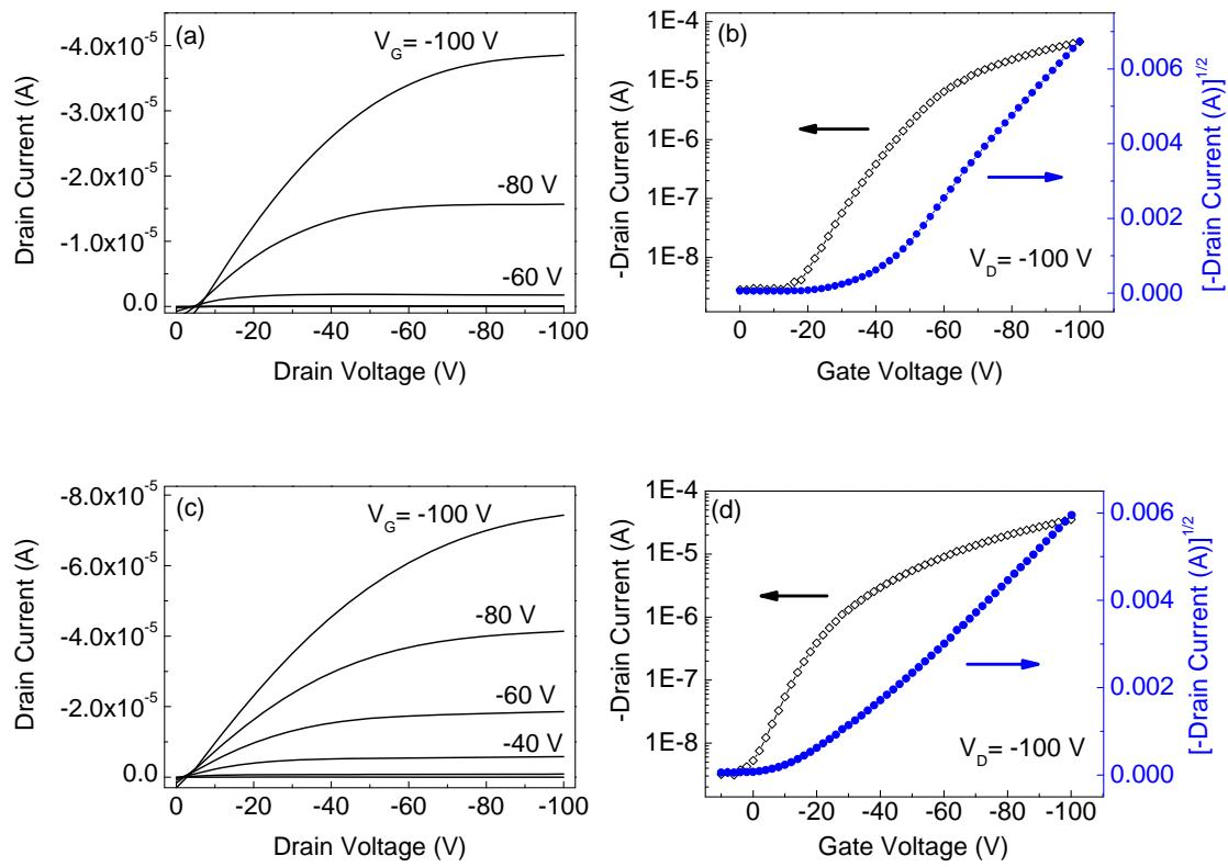
Fig. 5.  $I_D$ - $V_D$  characteristics and  $I_D$ - $V_G$  characteristics of (a, b) 4TC2P and (c, d) 4TC2Pme.
