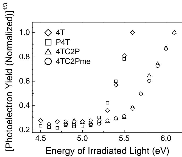
Fig. 2. Photoelectron emission yield spectra of materials.
