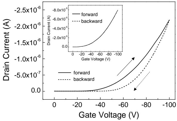
Fig. 6. Forward (solid line) and backward (dotted line)  $I_D$ - $V_D$  characteristics of 4TC2P OTFTs and (inset) 4TC2Pme OTFTs.
