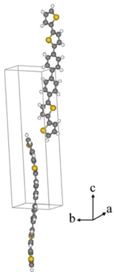
Fig. 4. 4TC2P unit cell. (Crystal class: monoclinic, Space group:  $P21$ , Cell Constants:  $a = 5.816 \text{ \AA}$ ;  $b = 7.2527 \text{ \AA}$ ;  $c = 25.2863 \text{ \AA}$ ;  $\beta = 96.265^\circ$ ; CCDC number: 673710, the crystallographic data can be obtained free of charge from the Cambridge Crystallographic Data Centre via [www.ccdc.cam.ac.uk/data\\_request/cif](http://www.ccdc.cam.ac.uk/data_request/cif).)
