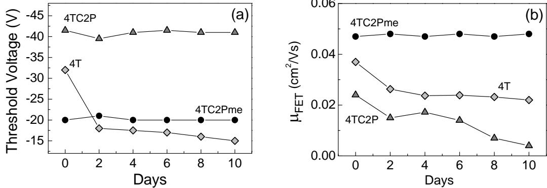
Fig. 7. Storage time dependences of (a) threshold voltage and (b) field-effect mobility of ( $\diamond$ ) 4T, ( $\blacktriangle$ ) 4TC2P, and ( $\bullet$ ) 4TC2Pme OTFTs.
