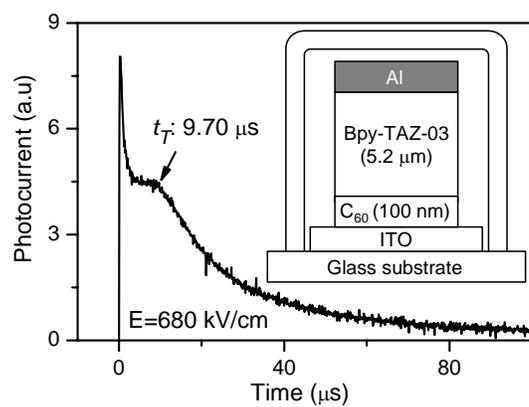
Figure 8. Electron transient photocurrent of TOF measurement of Bpy-TAZ-03 at the applied voltage of 360 V to the Al cathode. The inset shows device structure used.
