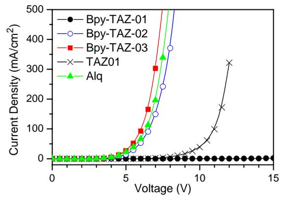
Figure 4. **Current density**-voltage characteristics of OLEDs with Bpy-TAZs as electron-transporting materials, showing together the reference devices with Alq and TAZ01
