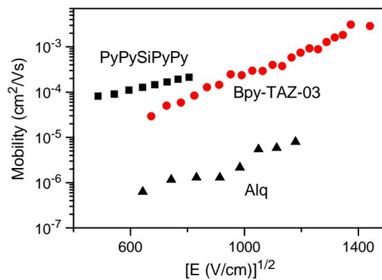
Figure 9. Electric field dependence of electron mobility of Bpy-TAZ-03, Alq, and PyPySiPyPy. Data for Alq and PyPySiPyPy were referred from the literature by Murata (see text).
