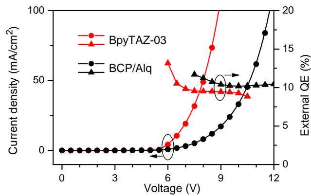
Figure 6.  $J$ - $V$  (left axis) and external quantum efficiency (QE)- $V$  (right axis) characteristics of the phosphorescent OLED with Bpy-TAZ-03 as a hole-blocking and electron-transporting material, showing together a reference device with the conventional structure.
