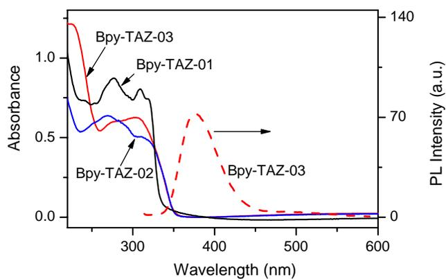
Figure 3. UV and visible absorption spectra of Bpy-TAZs thin-films. The thicknesses of the films are, respectively, 130 nm for Bpy-TZA-01, 90 nm for -02, and 90 nm for -3. PL spectrum of the Bpy-TAZ-03 film was also shown in the figure (right axis).
