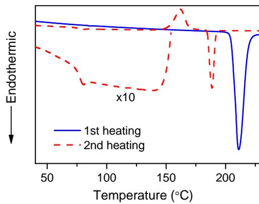
Figure 2. DSC curves of Bpy-TAZ-03 in first and second heating.
