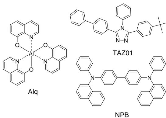
Figure 5. Device structure of OLEDs with different ET materials and chemical structures of materials used.
