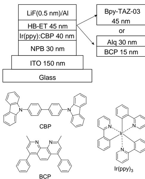
Figure 7. Device structure of phosphorescent OLEDs with Bpy-TAZ-03 as a hole-blocking and electron-transporting layer, and chemical structures of used other chemicals in the OLEDs.
