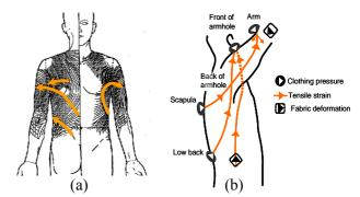
**Fig.3** Wrinkles of skin around the shoulder joint. [12] (a) Wrinkle pattern of the skin around the shoulder joint. (b) Tensile strain model base on the wrinkle pattern of skin.
