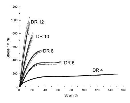
Figure 8. Stress-strain curves of the neck-drawn PP fibers.
