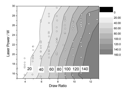
Figure 2. Drawing stress of PP as a function of laser power and draw ratio. Numeral 20 to 140 in the figure indicates drawing stress in MPa.
