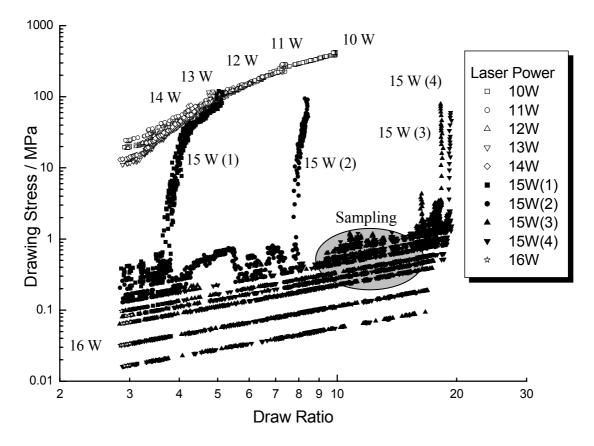
Figure 3. Neck drawing and flow drawing of PP. The drawing stress as a function of laser power and draw ratio is shown.
