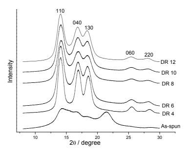
Figure 6. WAXD profiles of as-spun and neck drawn PP fiber.
