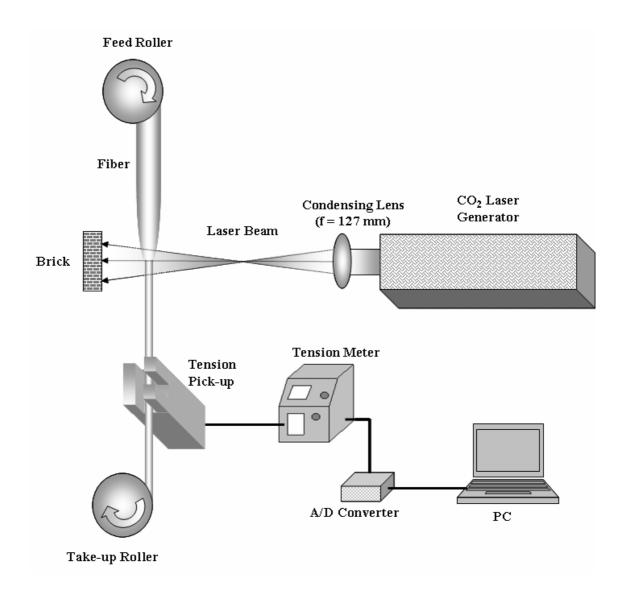
Figure 1a. Schematic diagram of the CO<sub>2</sub> laser-heated-drawing system.
