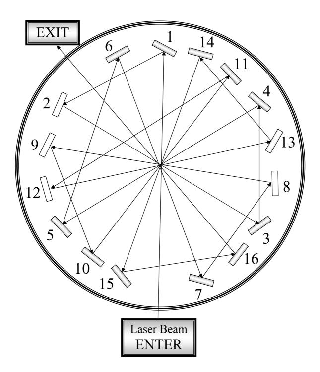
Figure 1b. Schematic diagram (top view) of the multidirectional laser irradiation system. Number 1 to 16 represents corresponding mirror where laser beam is reflected successively. Fiber is run vertically through the centre point of each reflection.
