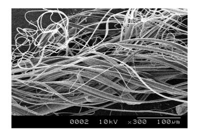
Figure 7. SEM image of fractured fibrillated PP (draw ratio 12) fiber.
