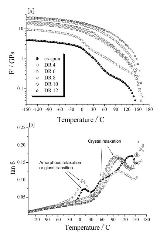
Fig. 9. (a) Storage modulus (E') and (b) loss tangent (tan  $\delta$ ) curves of as-spun and neck drawn PP fibers.
