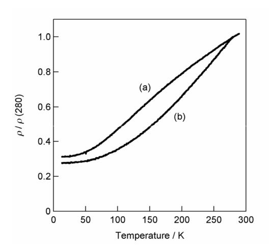
Figure 1. The normalized resistivity as a function of the temperature for sintered pellets of (a) layered  $K_{0.2}RuO_{2.1}$  and (b) rutile-type  $RuO_2$ .
