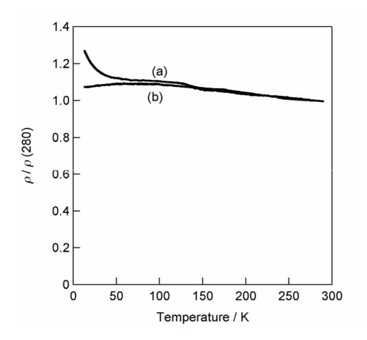
Figure 2. The normalized resistivity as a function of the temperature for non-sintered pellets of (a) layered  $H_{0.2}RuO_{2.1}$  and (b)  $RuO_2 \cdot nH_2O$ .
