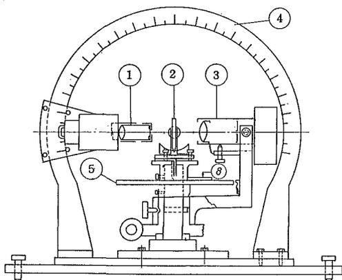
Fig. 1 Lateral view of 3-Dimensional Goniophotometer (GP-meter)
