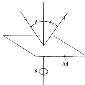
Fig. 2 Relation of incidence angle ( $\phi_i$ ) and reflection angle ( $\phi_r$ ) with rotation of angular disk (Ad)
