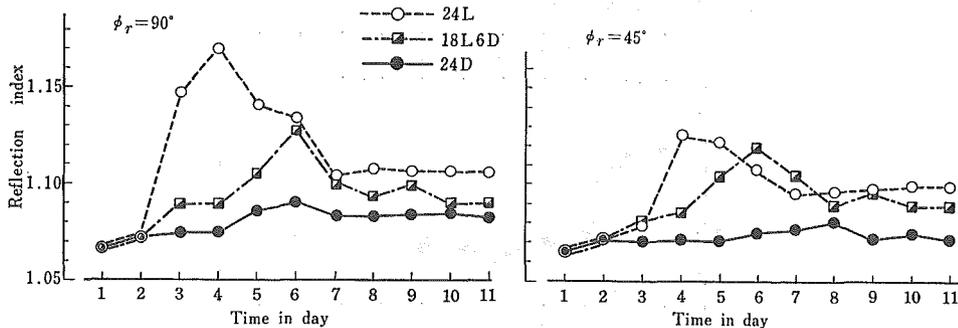
Fig. 12 Change of reflection index in each regime measured by GP-meter
