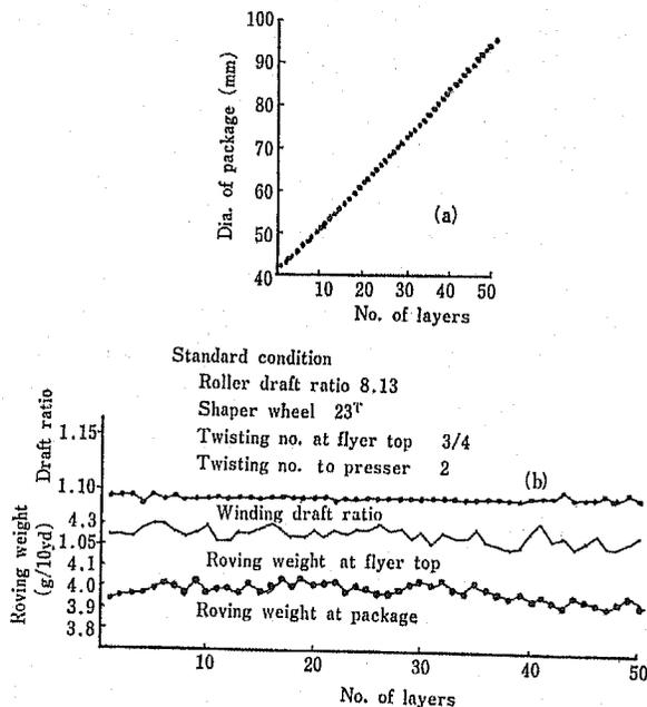
Fig. 5 Standard winding
