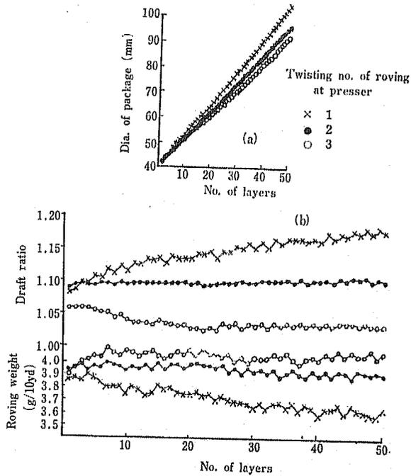
Fig. 7 Effects of twisting no. to presser
