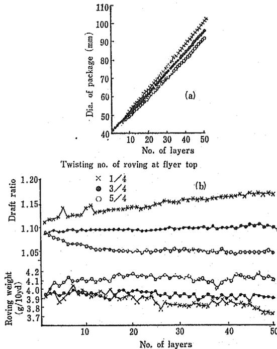
Fig. 6 Effects of twisting no. at flyer top
