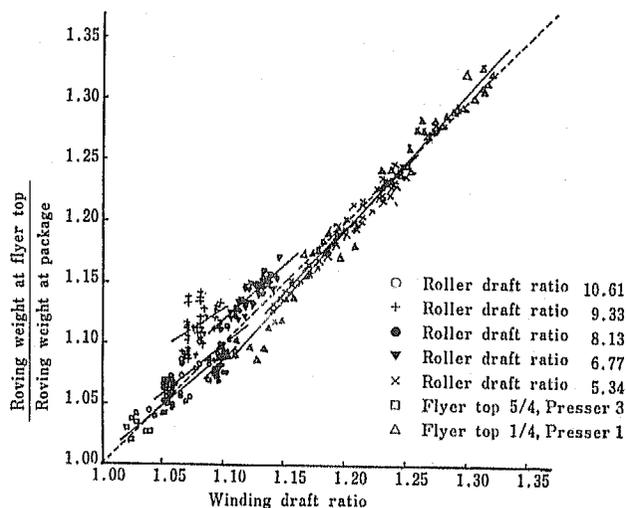
Fig. 13 Correlation between winding draft and roving weight
