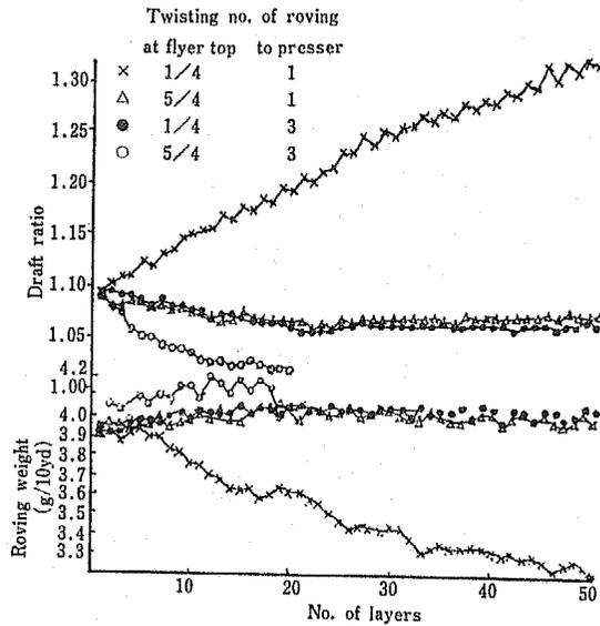
Fig. 8 Effects of twisting no. at fly top and to presser
