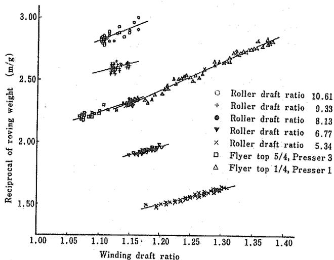
Fig. 12 Relations between winding draft and roving weight
