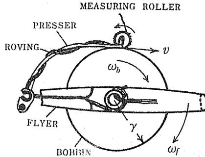
Fig. 1 Winding part and measuring roller
