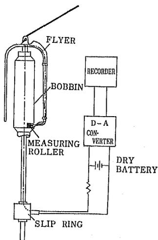
Fig. 3 Measurement system of winding speed
