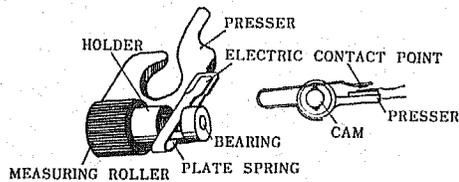
Fig. 2 Measuring roller
