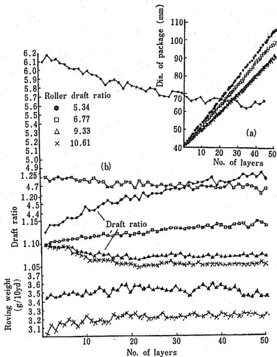
Fig. 11 Effects of roller draft ratio
