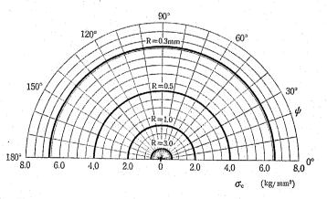
Fig 9. Diagram of the stress  $\sigma c$  on the apparent central fiber
