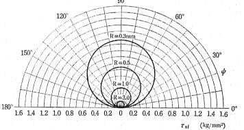
Fig 8. Diagram of the bending stress  $\sigma_{sf}$  and the torional stress  $\tau_{sf}$  on the fill side fiber.
