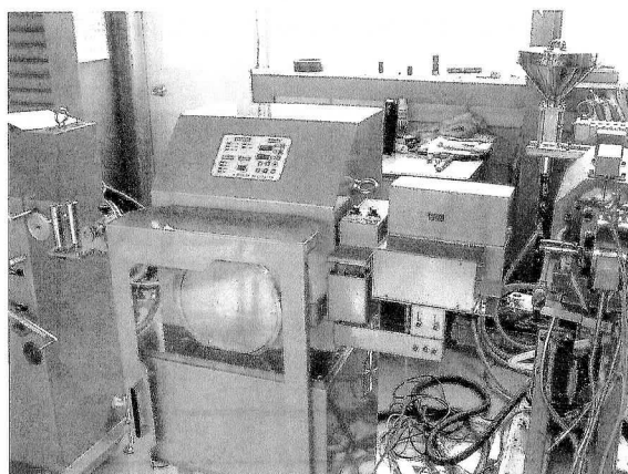
Fig.6 Non-contact temperature measuring system installed in the electric wire production system.
