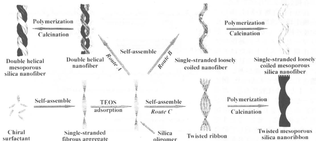
Figure Schematic representation of formation of different kinds of silica nanostructures.
