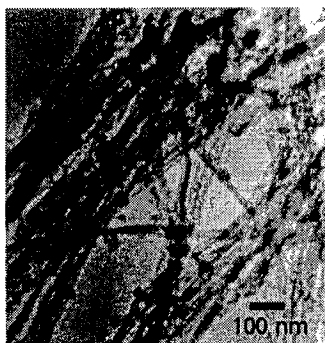
Figure 1: TEM image of carbon nanotubes prepared by template carbonization method using mesoporous silica.
