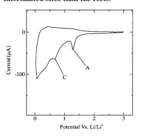
Fig.2. CV of heat-treated (at  $1000^{\circ}$ C) MWNT (1<sup>st</sup> cycle) at a sweep rate of 0.1 mVs<sup>-1</sup>.
