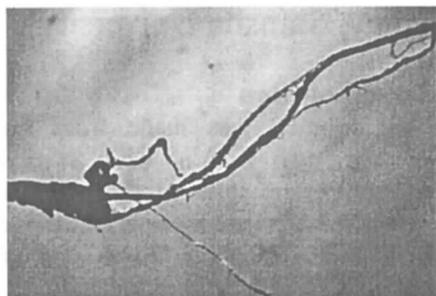
Figure 2. Fiber Fibrillation
