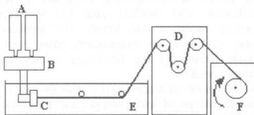
A: Spinning solution reservoir, B: Gear pump, C: Nozzle, D: Feed roller, E: Coagulation bath
