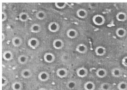
Figure 3. Phase Separation of PVA Film
