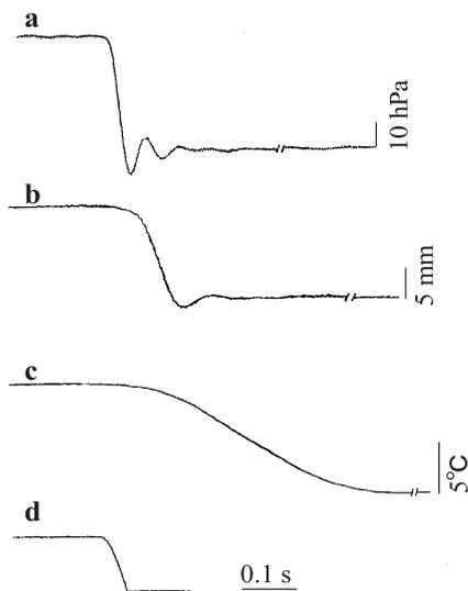
**Fig. 4** Typical examples of time constants of sensor responses in measuring system
