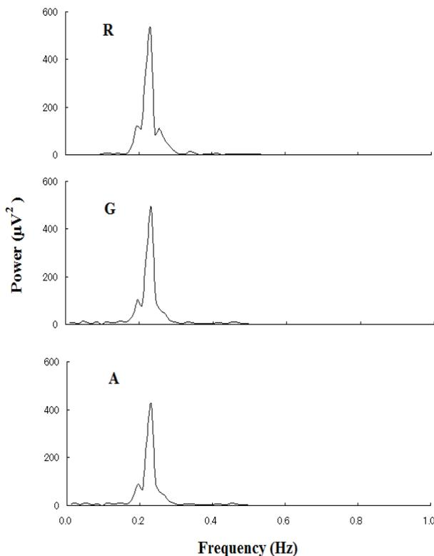
**Fig. 6** Power spectra of the 3 waves (respiration, girth of abdomen, and waistband-pressures shown in Fig. 5). Legends of R, G, and A correspond to those of Fig. 5. Subject E
