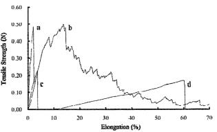
Fig. 3. The strength and elongation curves of several silk protein materials. (a) Solid silk protein gland. (b) Spun silk net. (c) Drawn solid silk protein without gland. (d) Solid silk protein. a, b, and c were measured in dry state, d was measured in wet state.
