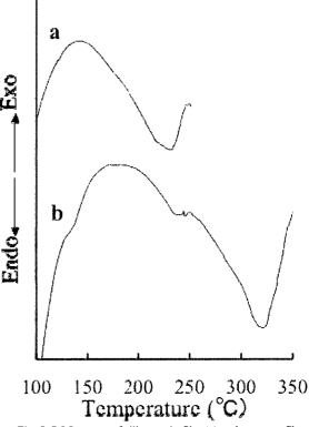
Fig. 5. DSC curves of silk protein film (a) and spun net fiber (b)
