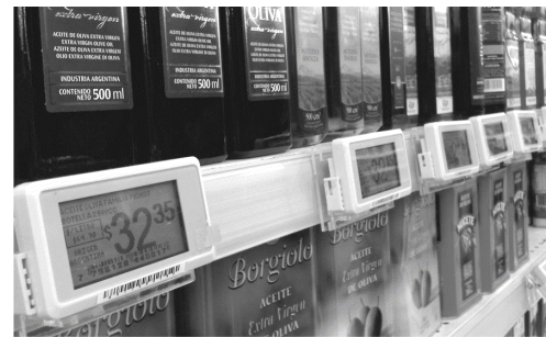
Fig. 1. A sample photograph of the ESL system. (By courtesy of Optoelectronics Co., Ltd.)
