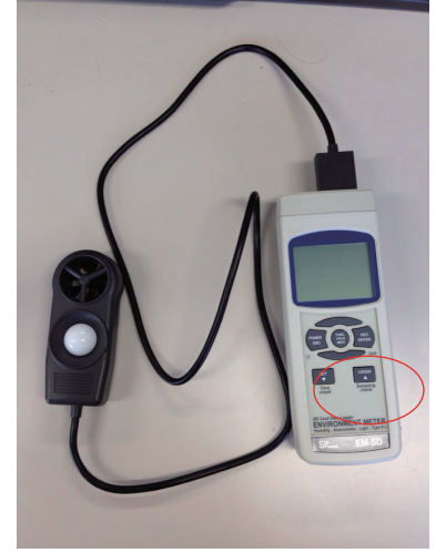
(b) Sensor of temperature and logger
