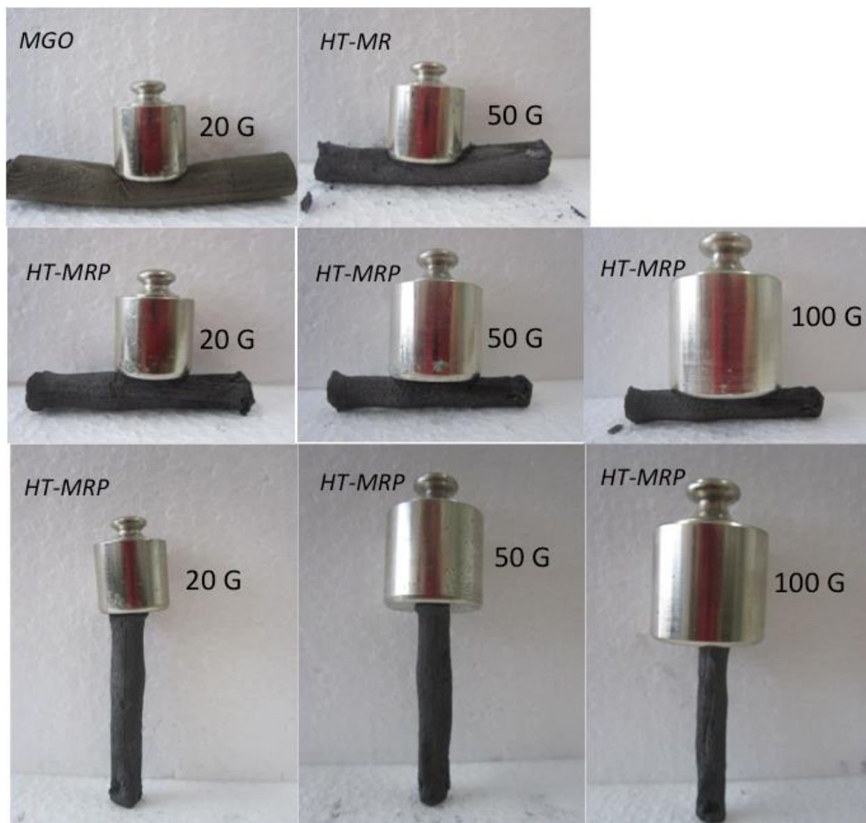
Figure 2. Comparison of the strength of the initial and modified monoliths. The diameter of HT-MRP monolith is 7 mm.
