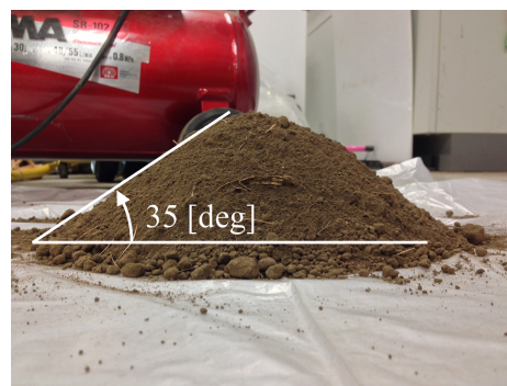
Fig. 13 The angle of repose in the experiment.
