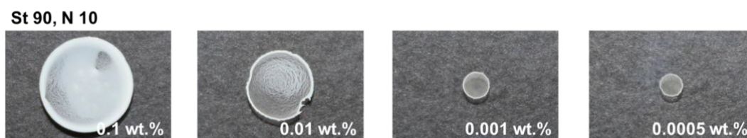
Figure 1-2-19. Dried structure of core particle dispersions. The dispersions were dried at room temperature.
