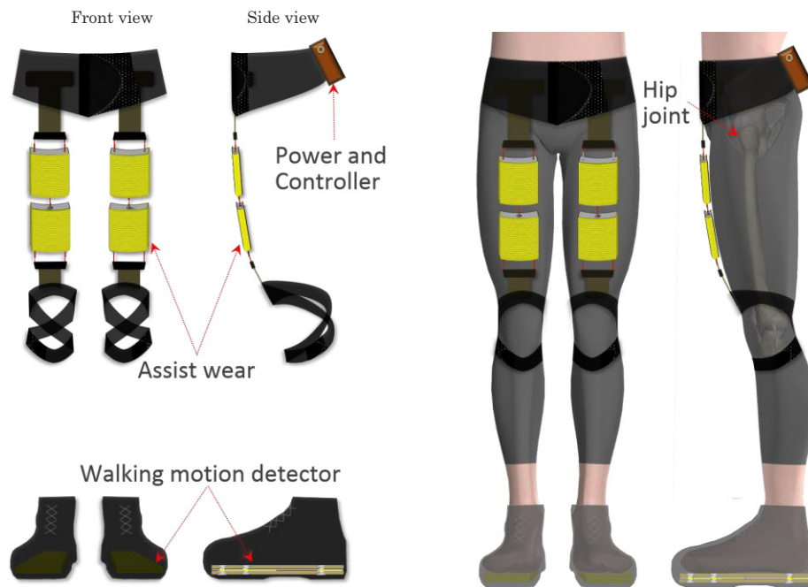
Fig. 3.2.1. Structure of the proposed walking assist wear with PVC gel artificial muscles.
