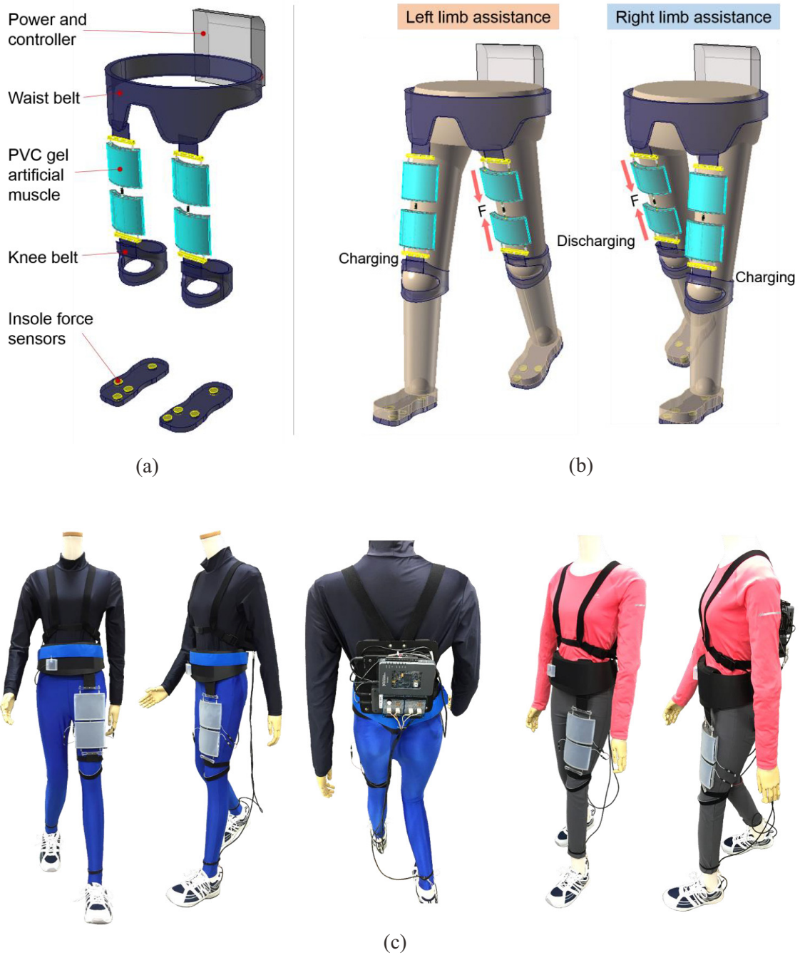
Fig. 4.4.1. Prototype of the walking assist wear with PVC gel artificial muscles. (a) Overview of a 3D model of the prototype. (b) Mechanism of assistance. (c) Overview of the real fabricated prototype, wearing on a model.
