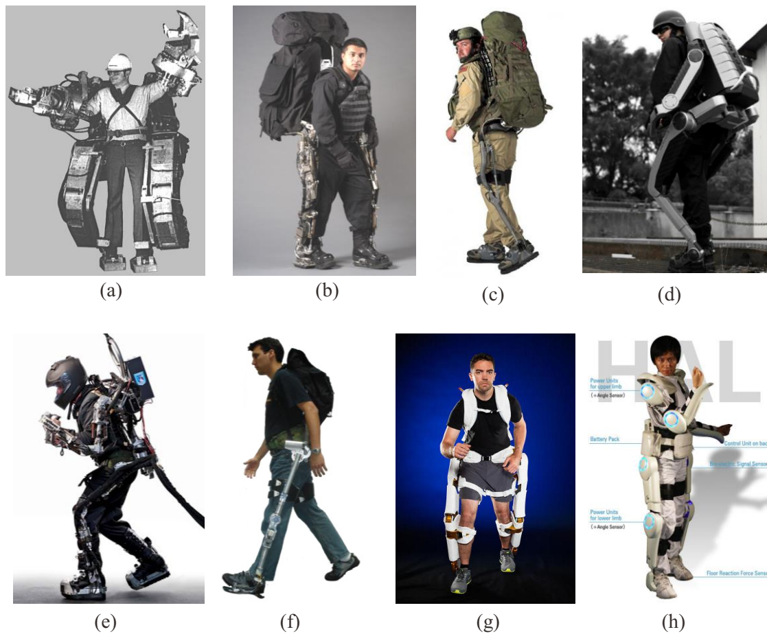
Fig. 1.2.1. Exoskeletons for human augmentation. (a) General Electric’s Hardiman exoskeleton [19]. (b) The University of California at Berkeley’s BLEEX exoskeleton [21]. (c) The Berkeley Robotics and Human Engineering Laboratory’s ExoHiker™ robotic exoskeleton [24]. (d) French engineering company RB3D’s Hercule exoskeleton [25]. (e) Raytheon Sarcos’s XOS exoskeleton [26]. (f) MIT’s lower limb exoskeleton [27]. (g) NASA X1 exoskeleton [28]. (h) The Cyberdyne Inc.’s HAL exoskeleton [29].
