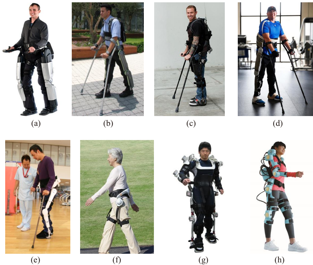
Fig. 1.2.2. Robotic wears and exoskeletons for rehabilitation, medical assistance. (a) The New Zealand REX Bionics Ltd.’s REX exoskeleton [31]. (b) Argo ReWalk™ exoskeleton [32]. (c) The Berkeley Bionics’ eLEGS exoskeleton [33]. (d) Vanderbilt’s exoskeleton [34]. (e) The Cyberdyne Inc.’s HAL exoskeleton for rehabilitation [30]. (f) Honda’s robotic device [35]. (g) The Toyota Technological Institute’s exoskeleton [36]. (h) The ShinShu University’s robotic wear CURARA® [37].
