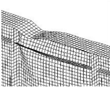
Figure 5. Deformation pattern for  $b=1200$  mm &  $t_f=15$ mm
