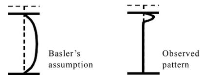
Figure 9 Observed and assumed deformation patterns
