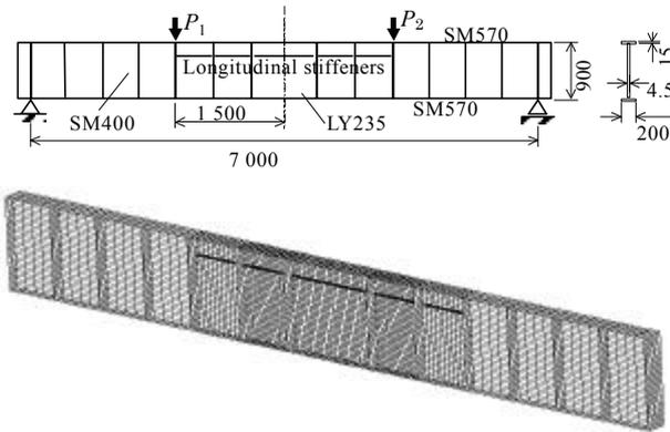
Figure 3. Example of the model layout and FEM mesh pattern
