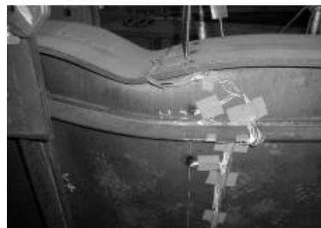
Figure 1. Observed flange vertical buckling
