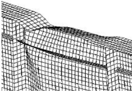
Figure 6. Deformation pattern for  $b=1200$  mm &  $t_f=14$ mm
