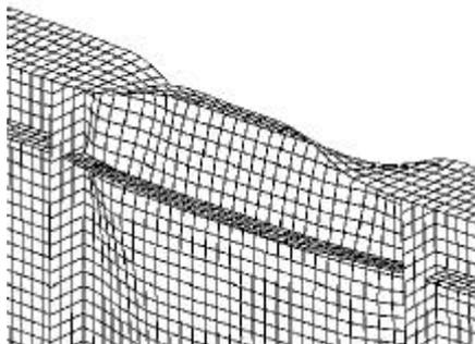
Figure 7. Deformation pattern for  $b=1200$  mm &  $t_f=13$ mm
