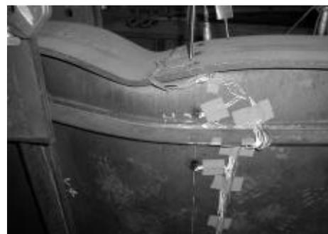
Figure 1. Observed flange vertical buckling
