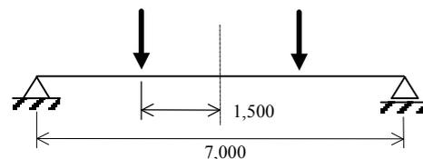
Figure 2. Loadings of experimental test
