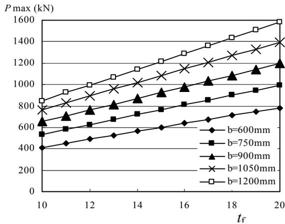
Figure 8 Peak load according to flange thickness
