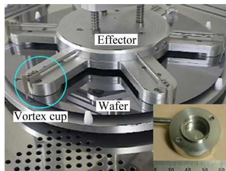
Figure 2. Non-contact handling system using vortex cups. [12].
