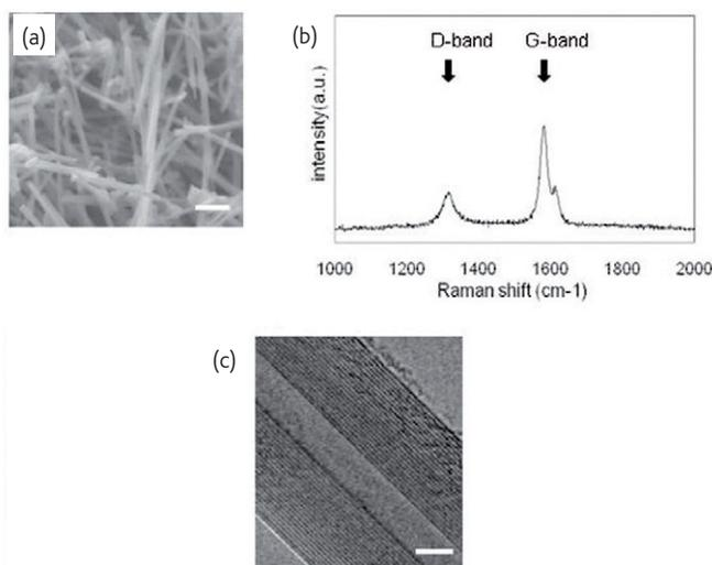
**Fig. 2** Characterization of MWCNTs. (a) SEM images of MWCNTs revealed a fibrous morphology with an approximate diameter and length of 100 nm and 10  $\mu\text{m}$ , respectively. Scale bar, 400 nm. (b) Raman spectra of MWCNTs. (c) TEM images of MWCNTs revealed multiple walls. Scale bar 5nm.
