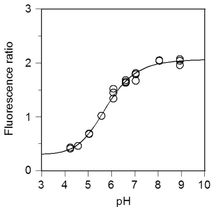
**Fig. 1** *In vitro* standard pH calibration curve of 6-CF. The fluorescence ratio (open circles) of 488 nm- and 458 nm-excited images was calculated for each CF solution at various pH values. Solid line shows a sigmoidal curve fitted by the following equation: fluorescence ratio =  $0.30 + 1.77 / [1 + (pH/5.79)^{-9.05}]$  ( $r^2 = 0.993$ ).
