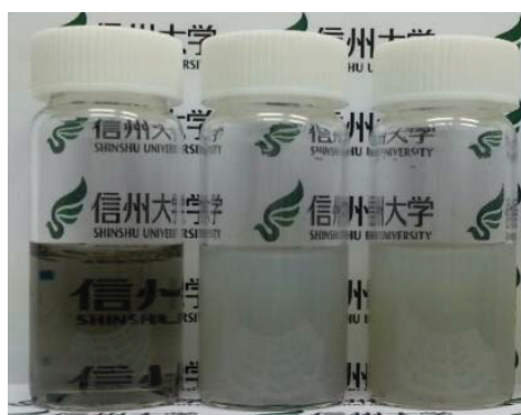
Figure 4.3.3 The ultracentrifugated semitransparent D-DW suspension (left), the following addition of MAP to D-DW suspension (middle) and after adding 20 μl of FeCl 3 solution (100mM) to MAP-DW suspension.
