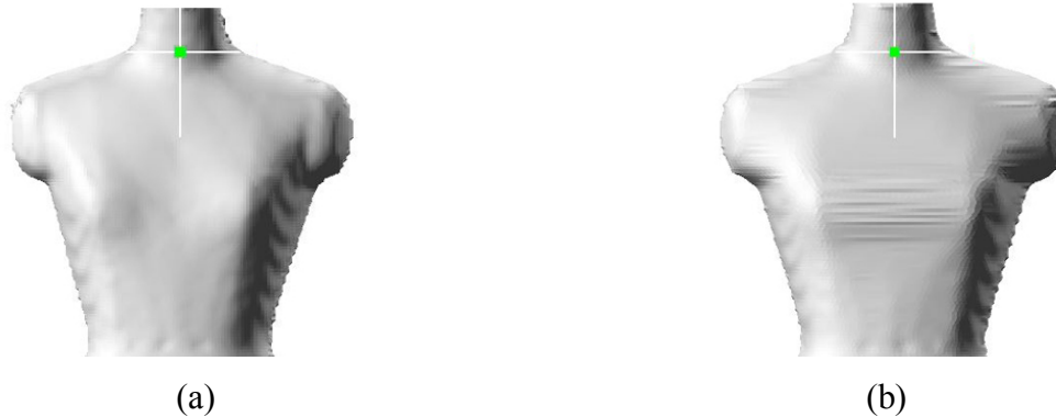
Figure 3.6 Process of convex hull at bust part: (a) Scanned bust; (b) Bust reconstructed with convex hull
