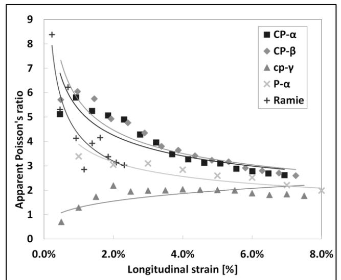
Figure 12 Relationship between apparent Poisson's ratio and the longitudinal strain of spun yarn samples; CP- $\alpha$ , CP- $\beta$ , CP- $\gamma$ , P- $\alpha$  and Ramie
