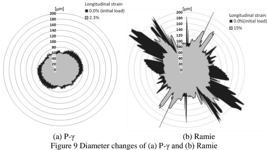
Figure 9 Diameter changes of (a) P- $\gamma$  and (b) Ramie
