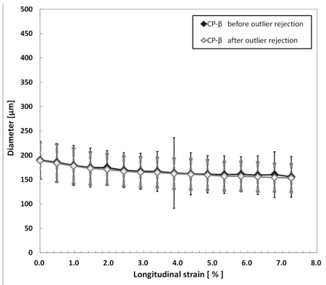
Figure 5 Relationships between diameter and longitudinal strain of CP-β before and after outlier rejection
