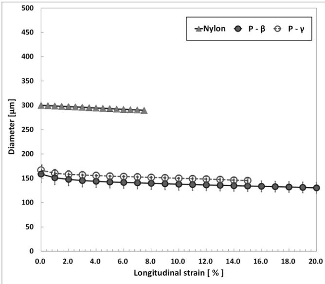
Figure 3 Relationships between diameter and longitudinal strain for P-β, P-γ and Nylon samples
