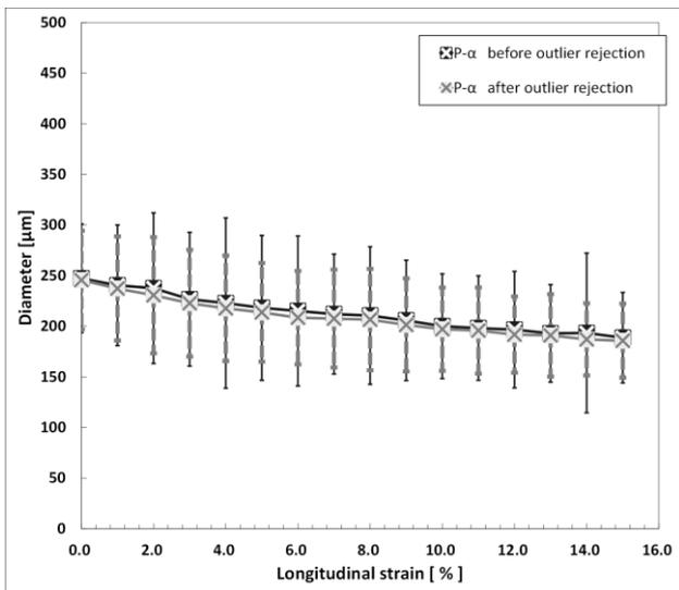
Figure 7 Relationships between diameter and longitudinal strain of P-α before and after outlier rejection
