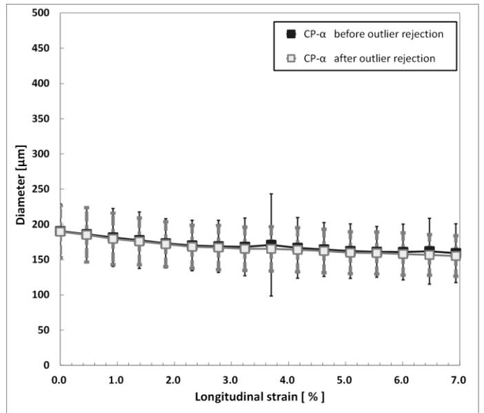
Figure 4 Relationships between diameter and longitudinal strain of CP-α before and after outlier rejection
