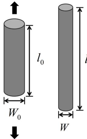
Figure 1 Changes in elongation and diameter in the longitudinal direction
