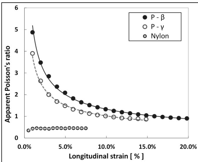
Figure 11 Relationship between apparent Poisson's ratio and the longitudinal strain of filament yarn samples; P- $\beta$ , P- $\gamma$  and Nylon
