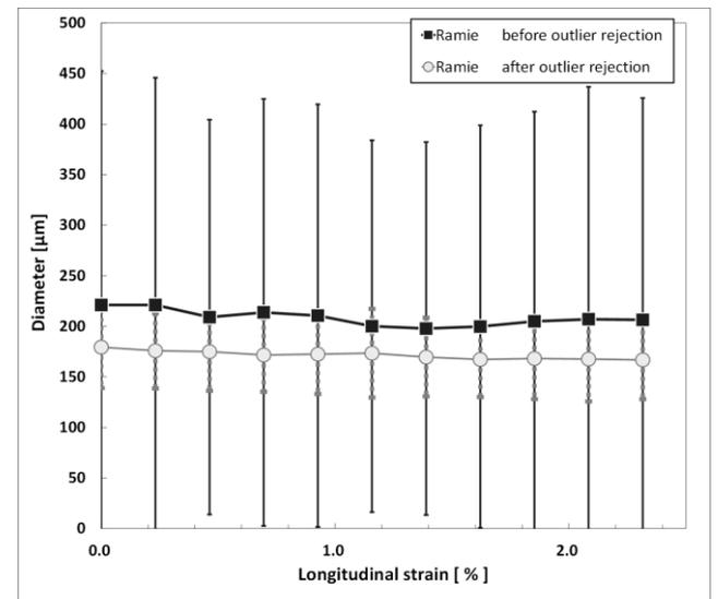
Figure 8 Relationships between diameter and longitudinal strain of Ramie before and after outlier rejection
