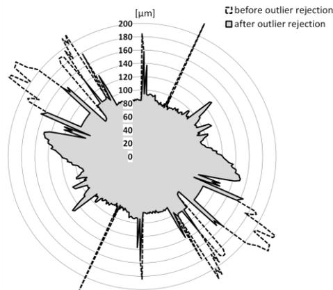
Figure 10 Example of outlier rejection result for Ramie at initial load
