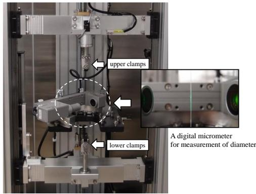
Figure 2 Apparatus for the measurement of the yarn diameter in tension.
