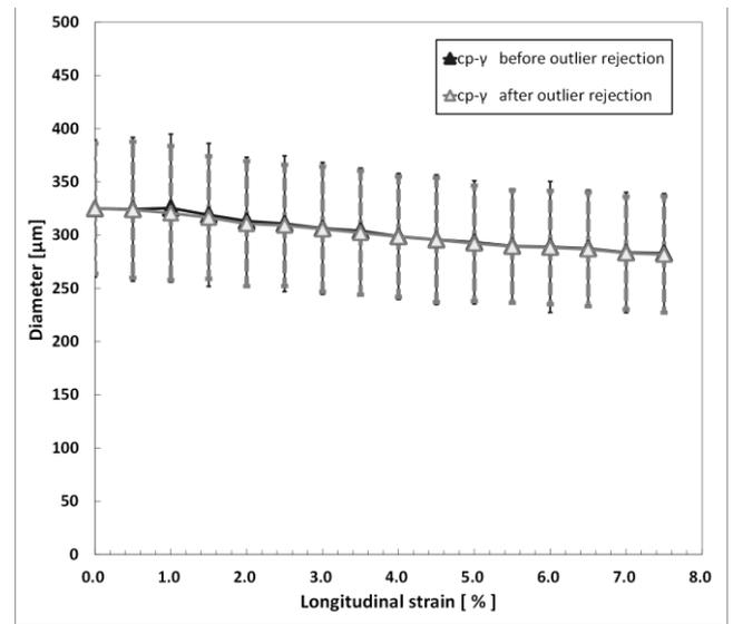
Figure 6 Relationships between diameter and longitudinal strain of CP-γ before and after outlier rejection
