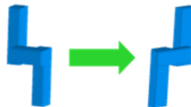
Fig. 2 Orientational changes of molecules by electric field [A] in a uniaxial nematic ( N_u ) phase and [B] in biaxial nematic ( N_b ) phases of (a) board-like molecules, (b) banana-shaped molecules and (c) crank-like molecules.
