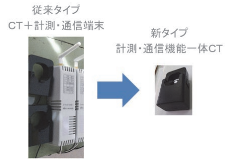
Fig. 2 Wireless current sensor without battery.
