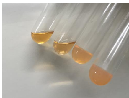
Figure 2.3 Photographs of samples. The solvents are chloroform (solution), DMF (solution), PC (gel), and \gamma -BL (gel) from right to left.
