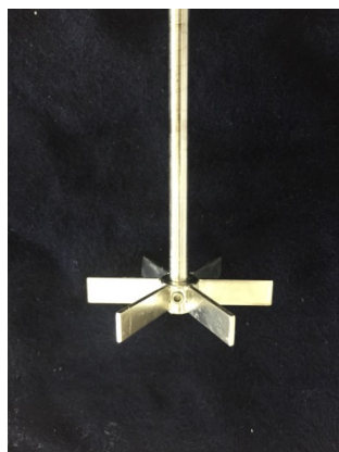
Fig. B.2 Photograph of the stirring blade used in the experiment.
