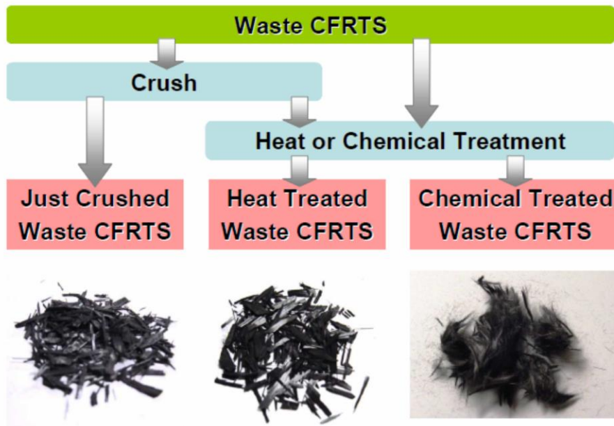
Fig. 1-8 Pretreatment of CFRP recycling, crush, heat treatment and chemical treatment 34) .
