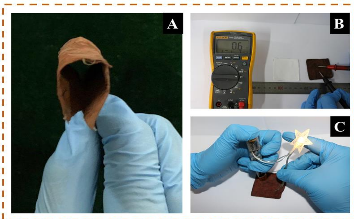
Figure 6. (A) Flexible N6 NFs (B) resistance measurement of copper-coated N6 NFs after ELD process (C) conductivity of N6 NFs.
