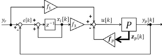
Fig. 6. Servo system with rotational and expansionary coordinate transformations
