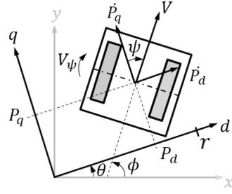
Fig. 2. Vehicle model with the rotational coordinate transformation
