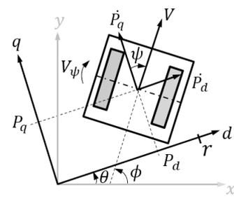
Fig. 2. Vehicle model with the rotational coordinate transformation
