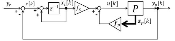
Fig. 3. Servo system with the rotational coordinate transformation
