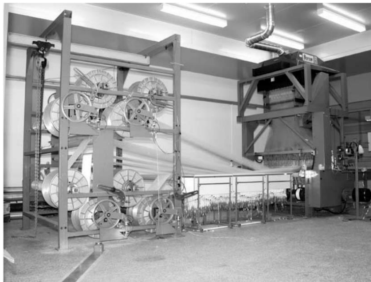
Fig. 1-3. Jacquard loom used to weave 3D woven fabric[40].
