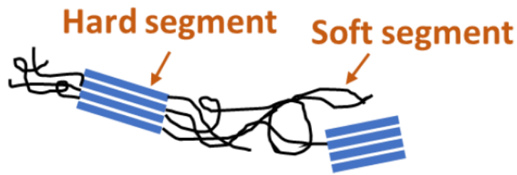
Figure 1-5. Schematic of TPU structure
