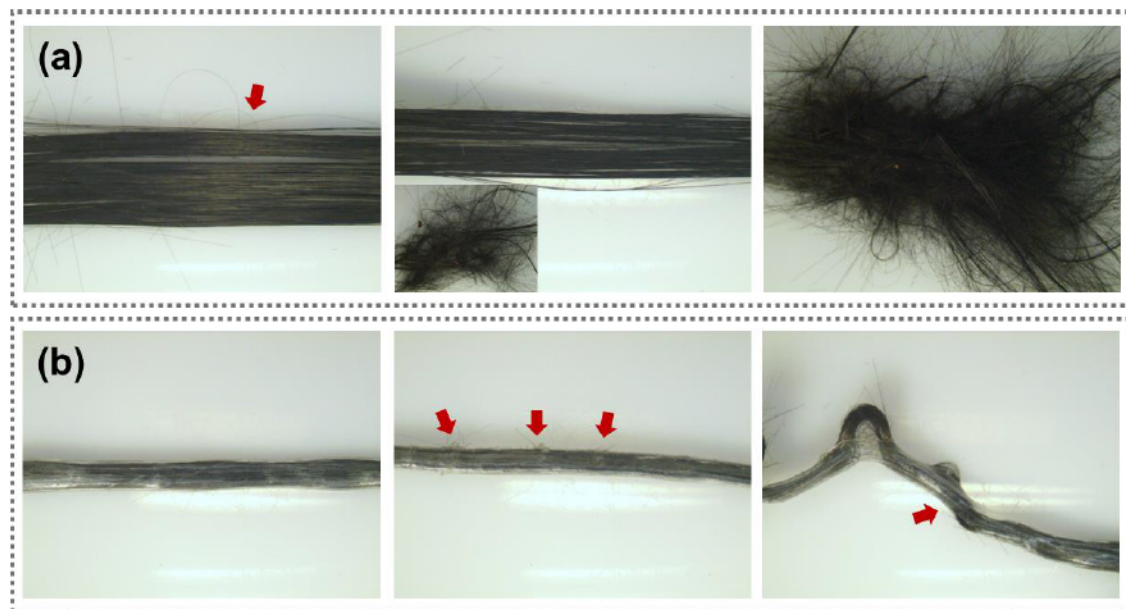
Figure 2-4. Images of the friction of the (a) original and (b) TPU-wrapped carbon fiber tows.
