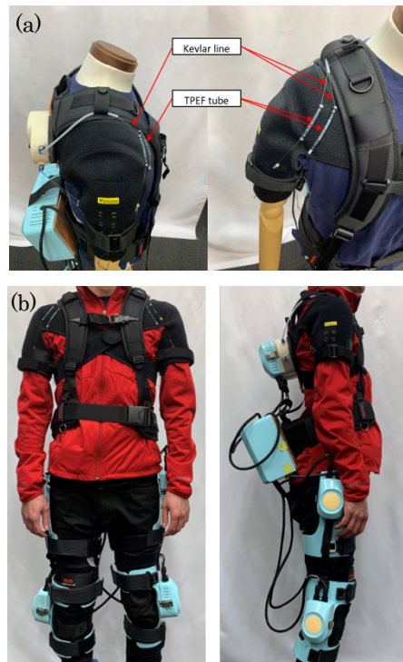
図 2 (a)Side and back views of the spool mechanism and the assist wear mounted on the torso. (b)Coordinated motion support system of paralyzed upper and lower limbs.
