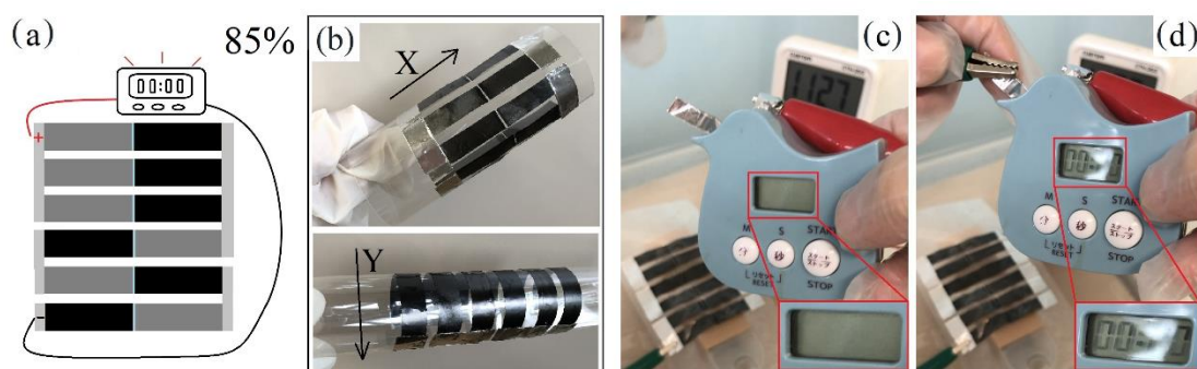
Figure 2-8 (a) The schematic of 6-HEGs in expansion, (b) the digital photo of 6-HEGs under bending, (c-d) the digital photos of 6-HEGs to power a timer ( V > 1.5 V, I > 25 \mu A) under 85%
