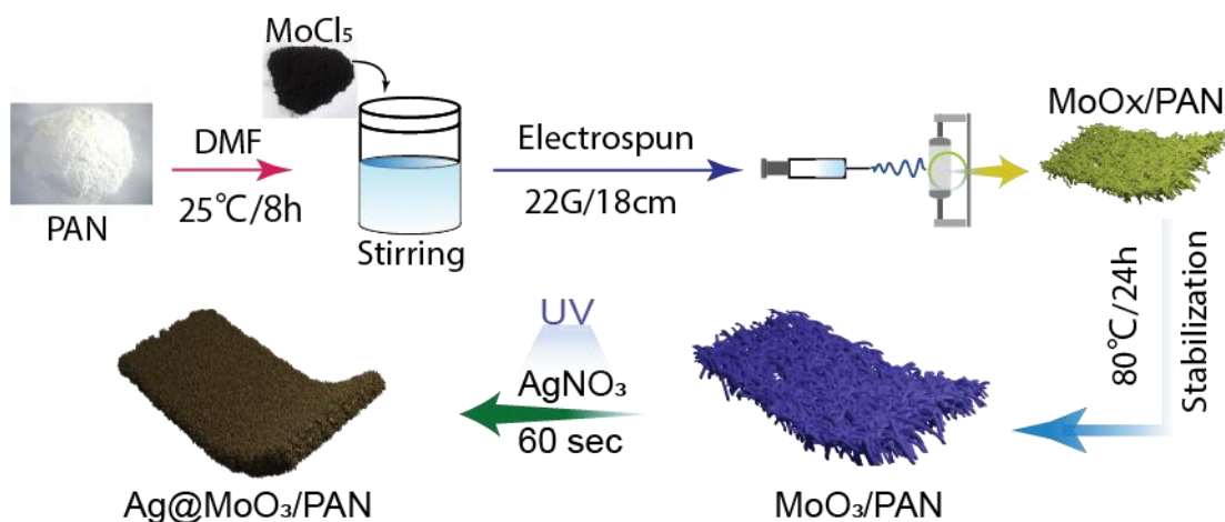
Figure 3—2: Graphical illustration of \text{MoO}_3/\text{PAN} membrane synthesis and \text{Ag}@\text{MoO}_3/\text{PAN} membrane fabrication.
